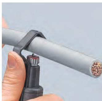
Setting the tool for circular cut
