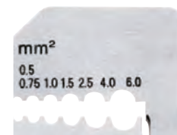
12 21 180: wire cross-sections in mm 2
