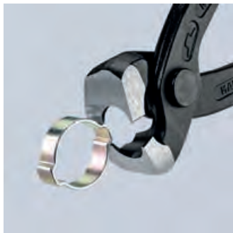
Using the front press nib
