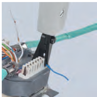
Inserts and cuts cables in one operation
