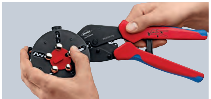
Changing the crimping dies: unlock the magazine position, take out the set of dies which the pliers have been pushed on
