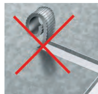
Notching without chip breaking
