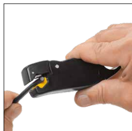
Inserting a coax cable
