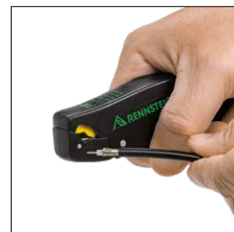
Stripping of 3 layers in one work step
