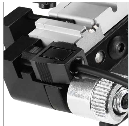
crimp the plug with the prepared cable in just one tool
