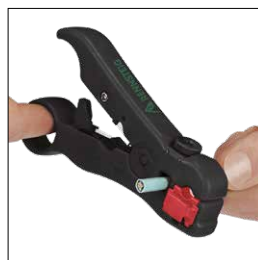
Stripping round data cables
