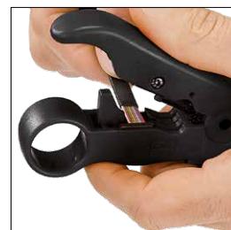
Stripping of flat cables
